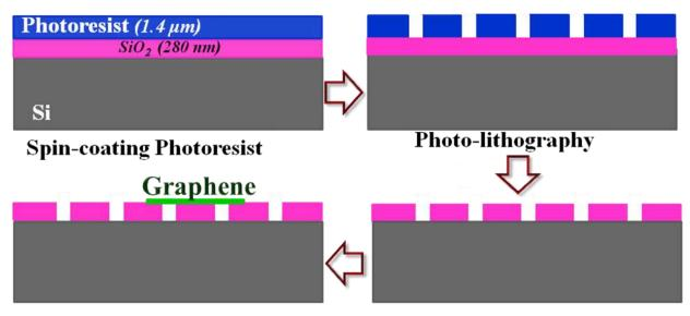
Micro-mechanical exfoliation Fabrication of suspended graphene sample
