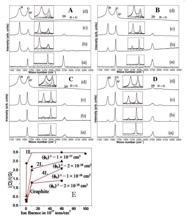
Fig. 3- Panel A-Raman spectrum from (a) pristine monolayer graphene and the same sample irradiated at fluences of (b)  $1 \times 10^{17}$  ions/cm<sup>2</sup>, (c)  $1 \times 10^{18}$  ions/cm<sup>2</sup> and (d)  $6 \times 10^{18}$  ions/cm<sup>2</sup>, panels B, C and D correspond to the same for a 2 layer graphene, 4 layer graphene and Graphite
