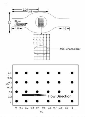
Figure 1 | (a) The model of braided bar constructed in a River Engineering Lab IIT Roorkee; (b) the sketch of the mid-channel bar model and measuring points (all dimensions in metres).
