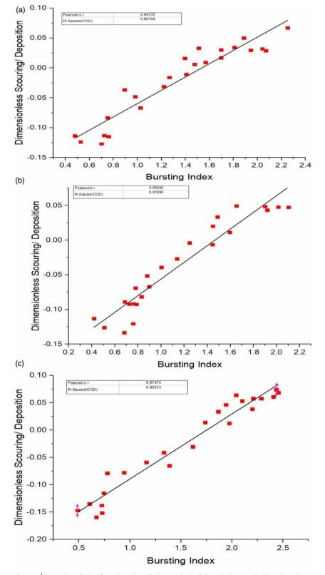
Figure 8 | (a)-(c) The variation of Bursting Index with the magnitude of dimensionless scouring/deposition that occurred in the vicinity of the mid-channel bar for the 1R, 2R and 3R experimental runs respectively.
