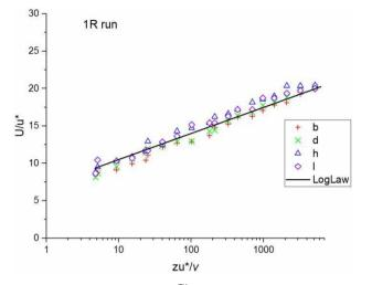
**Figure 2** | The variations of  $U/u_s$ , versus  $\frac{Zu_s}{9}$  for four different points located in the vicinity of the mid-channel bar.
