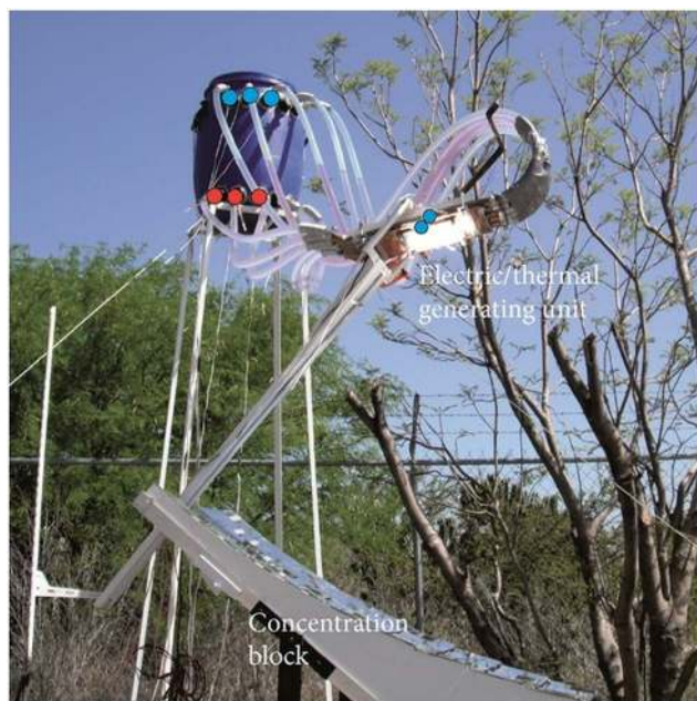
Fig. 5 Photograph of Parabolic Mirror with combined cogeneration of heat and electricity. Reproduced with permission from Hindawi: ref. 44 ©2013 Hindawi.
