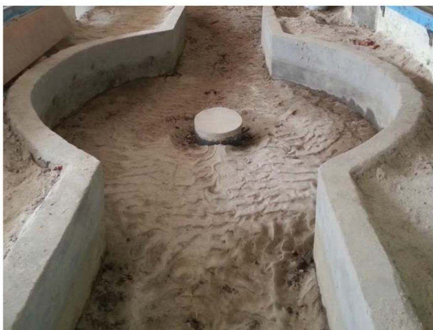
Figure 1. The mid-channel bar model constructed at River Engineering Lab (flume is 10 m long, 2.6 m wide, 1 m deep).
