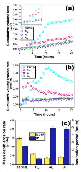
**Fig. 5.** (a) Cumulative volume loss, (b) cumulative erosion rate as a function of exposure time and (c) mean depth erosion rate and incubation period of  $Al_{0.1}$ CoCrFeNi, AlCoCrFeNi and  $Al_3$ CoCrFeNi complex concentrated coatings and conventionally used stainless steel 316L subjected to cavitation erosion. Inset in (a) shows the magnified view of the results during initial time period.
