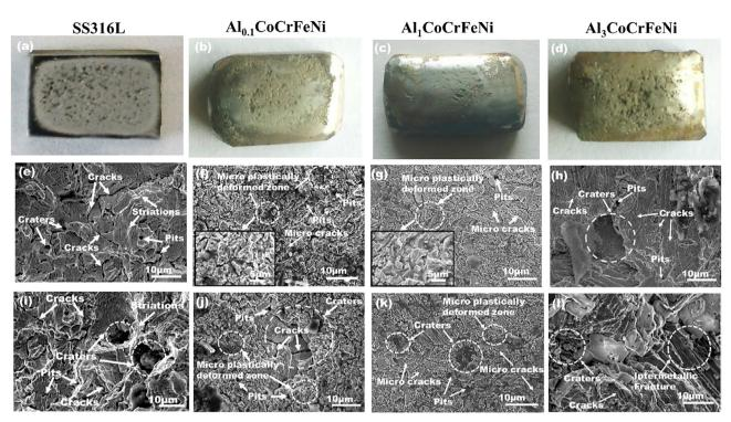
Fig. 11. Macrograph of (a-d) stainless steel and microwave synthesized Al<sub>x</sub>CoCrFeNi complex concentrated alloy coatings under cavitation erosion-corrosion condition for 20 h. The scanning electron micrograph images showing the surface morphology of the above samples subjected to cavitation (e-h) erosion and (i-l) erosioncorrosion testings. Insets in (f) and (g) show the micron scale TTS fracture of the coating during cavitation exposure.
