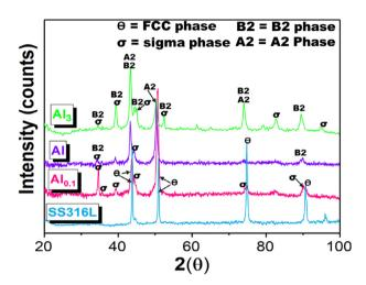
Fig. 1. X-ray diffraction (XRD) patterns of microwave derived  $Al_xCoCrFeNi$  (x = 0.1–3) complex concentrated coatings.
