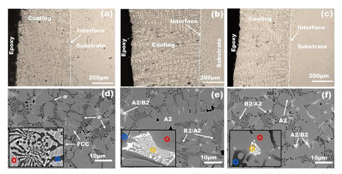
**Fig. 2.** (a-c) Optical and (d-f) scanning electron microscope image showing microstructure of the (a) and (d)  $Al_{0.1}$ CoCrFeNi, (b) and (e) AlCoCrFeNi and (c) and (f) coatings synthesized using microwave processing [25]. Insets show high magnification images of different phases. The composition of the phases is highlighted using different symbols and presented in Table 2.
