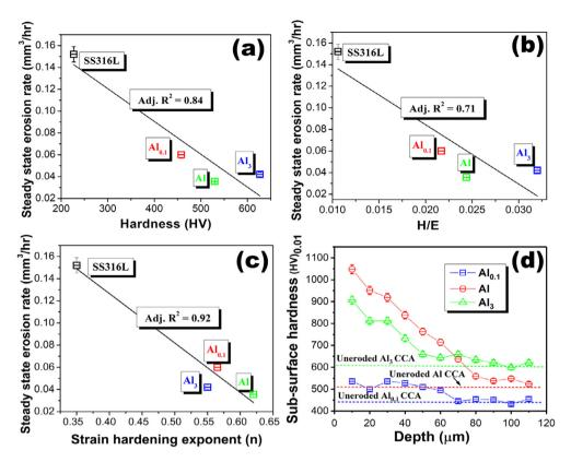
Fig. 6. The correlation of cavitation erosion rate of  $Al_{0.1}$ CoCrFeNi, AlCoCrFeNi and Al<sub>3</sub>CoCrFeNi complex concentrated coatings and stainless steel 316L with (a) hardness, (b) hardness to modulus ratio (c) strain hardening exponent (n) and (d) shows variation in sub-surface microhardness of the microwave derived  $Al_{0.1}$ CoCrFeNi, AlCoCrFeNi and Al<sub>3</sub>CoCrFeNi complex concentrated coatings under pure erosion.
