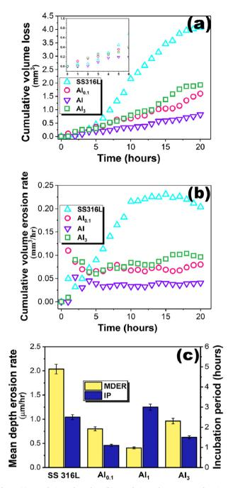
**Fig. 7.** (a) Cumulative volume loss, (b) cumulative volume rate as a function of exposure time and (c) mean erosion rate and incubation period of  $Al_{0.1}$ CoCrFeNi, AlCoCrFeNi and  $Al_3$ CoCrFeNi complex concentrated coatings and conventionally used stainless steel 316L subjected to cavitation erosion-corrosion in 3.5% NaCl solution. Inset in (a) shows the magnified view of the initial time duration.
