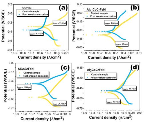
Fig. 9. The potentiodynamic polarization test results of the SS316L stainless steel and microwave synthesized AlxCoCrFeNi complex concentrated coating samples post cavitation erosion-corrosion testing. Control sample represents the test coupon not subjected to cavitation erosion.
