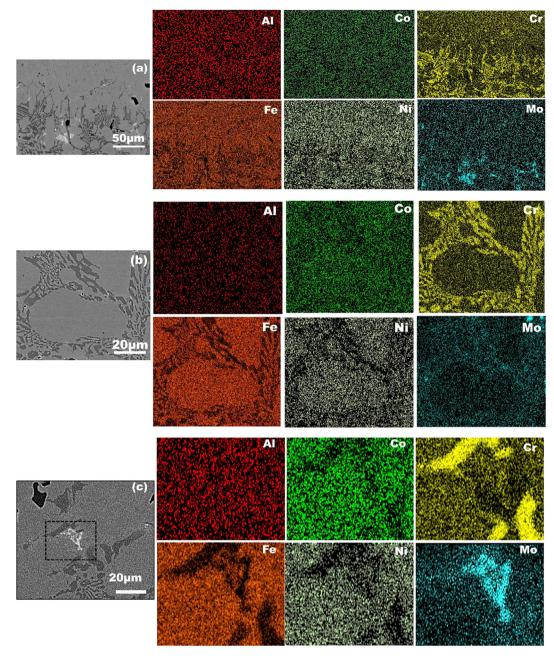
**Fig. 3.** Energy dispersive spectroscopy (EDAX) area maps showing the elemental distribution at the (a) interface of the coating and substrate (b) intercellular and intracellular region of Al<sub>0.1</sub>CoCrFeNi (c) Cr- and Mo-rich phases formed in AlCoCrFeNi coating.
