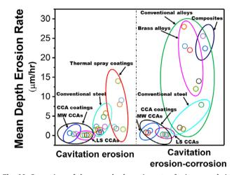
**Fig. 10.** Comparison of the mean depth erosion rate of microwave derived  $Al_{0.1}$ CoCrFeNi, AlCoCrFeNi and  $Al_3$ CoCrFeNi complex concentrated coatings with structural materials and conventional coating techniques subjected to erosion and erosion-corrosion conditions [12,13,37–41].
