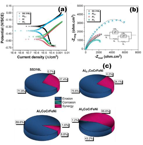
Fig. 8. (a) Tafel and (b) electrochemical impedance test (EIS) for microwave synthesized  $Al_{0.1}$ CoCrFeNi, AlCoCrFeNi and  $Al_3$ CoCrFeNi complex concentrated coatings with stainless steel using standalone electrochemical corrosion testing and (c) shows the percentage contribution of erosion. Corrosion and synergy calculated for the coatings and steel during cavitation erosion-corrosion testing.
