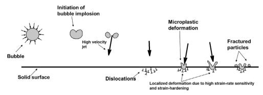
Fig. 12. Schematic illustrating the initiation of tearing topography surface (TTS) failure mode through microplastic deformation during cavitation erosion process for the complex concentrated alloys with high strain-rate sensitivity and strain hardening.
