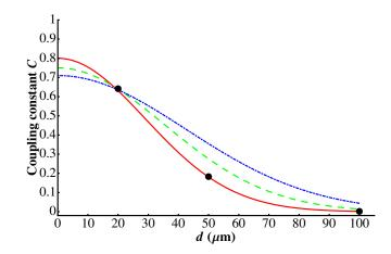
Fig. 4. Evolution of the coupling constant *C* versus spatial separation *d*. The filled circles are the measurements and the full lines are given by Eq. (12) with  $C_0 = 0.8$  and  $w_0 = 41 \ \mu m$  (full red line),  $C_0 = 0.75$  and  $w_0 = 50 \ \mu m$  (dashed green line), and  $C_0 = 0.71$  and  $w_0 = 60 \ \mu m$  (dot-dashed blue line)
