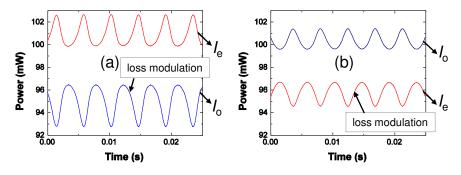
Fig. 2. Experimental results for a spatial separation  $d = 20 \ \mu m$ . (a) Evolution of the powers of the ordinary and extraordinary modes when the losses of the ordinary mode are modulated at 227 Hz. (b) Same as (a) when the losses of the extraordinary mode are modulated.
