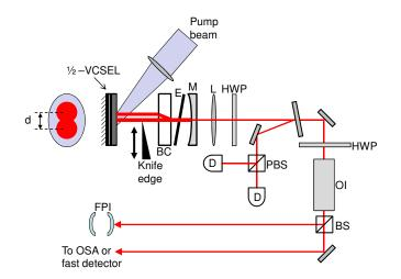
Fig. 1. Experimental setup. BC: birefringent crystal; HWP: half-wave plate; M: cavity mirror; E: étalon; FPI: Fabry-Perot interferometer. PBS: polarization beam-splitter; BS: beam splitter; L: lens; D: detector; OI: optical isolator; OSA: optical spectrum analyzer.
