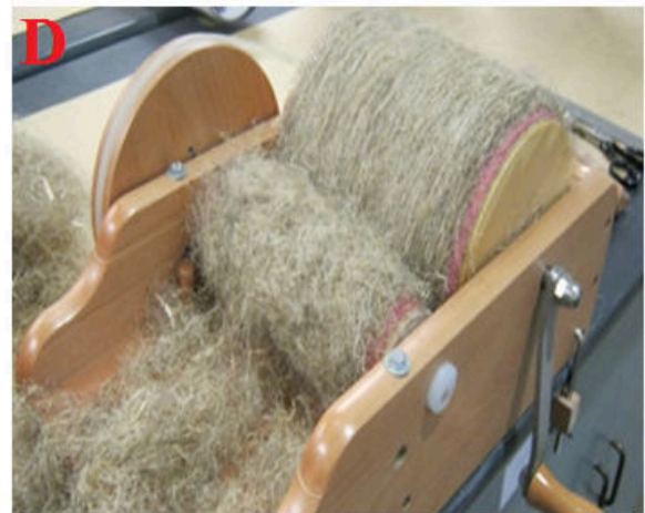
Figure 1. As received sisal fibre (A); as received hemp fibre (B); processing/ cleaning of hemp fibre in hot water (C) & carding of hemp fibres using hand carding machine (D)
