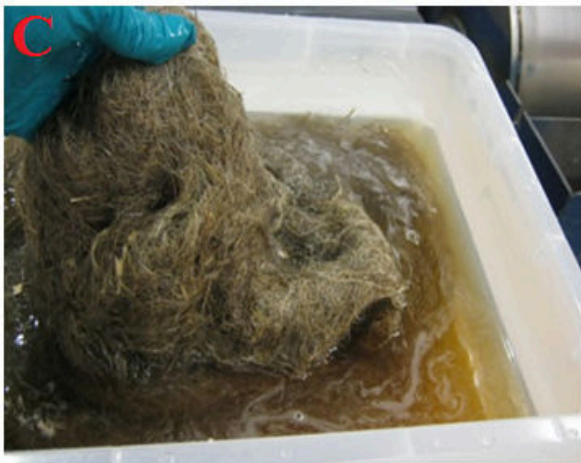
Figure 1. As received sisal fibre (A); as received hemp fibre (B); processing/ cleaning of hemp fibre in hot water (C) & carding of hemp fibres using hand carding machine (D)
