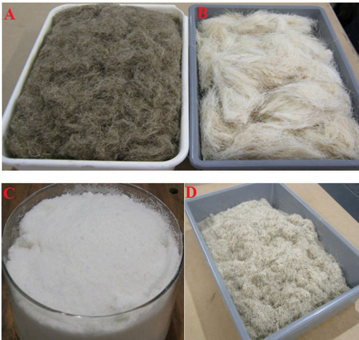
Figure 2. Processed hemp fibre (A); processed sisal fibre (B); Micronised PLA powder (C) & granulated hybrid natural fibres (Sisal fibre to Hemp fibre ratio 1:1 ratio) (D)
