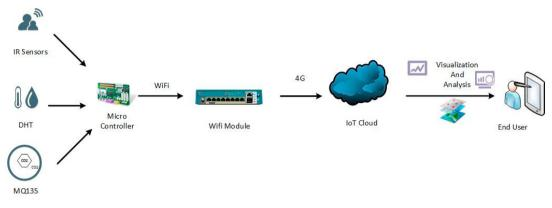
Fig. 1: Hardware architecture of the proposed cloud computing approach
