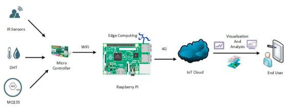
Fig. 2: Hardware architecture for the edge computing approach
