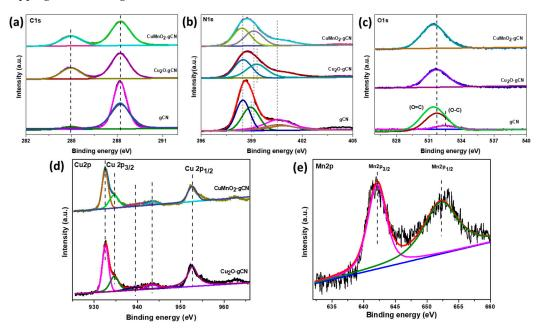
**Figure 4.** High-resolution X-ray photoelectron spectroscopy (XPS) spectra of (**a**) C1s, (**b**) N1s, (**c**) O1s, (**d**) Cu 2p, and (**e**) Mn 2p for gCN, Cu<sub>2</sub>O-gCN, and CuMnO<sub>2</sub>-gCN.
