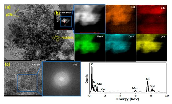
**Figure 2.** (a) Transmission electron microscopy (TEM), (b) STEM-HAADF images of CuMnO<sub>2</sub>-gCN and corresponding EDX elemental mapping of the selected area in (b,c) HRTEM image of CuMnO<sub>2</sub>-gCN and corresponding fast Fourier transform (FFT) pattern of the selected area.
