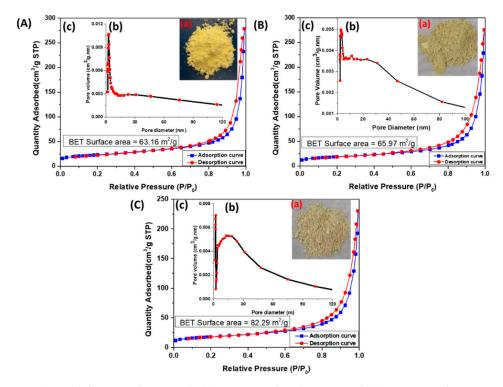
**Figure 5.** (**A**–**C**) The optical images (**a**,**b**) pore size distribution, and (**c**) nitrogen adsorption and desorption isotherms of gCN, Cu<sub>2</sub>O-gCN, and CuMnO<sub>2</sub>-gCN, respectively. BET, Brauner–Emmet–Teller.
