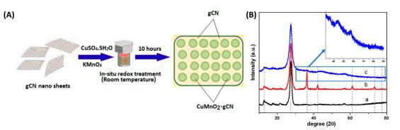
**Figure 1.** (**A**) Schematic representation of the catalyst synthesis. (**B**) X-ray diffraction (XRD) pattern of (**a**) graphitic carbon nitride (gCN), (**b**) Cu<sub>2</sub>O-gCN, and (**c**) CuMnO<sub>2</sub>-gCN.
