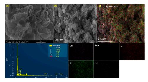
**Figure 3.** (**a**,**b**) Scanning electron microscopy (SEM) images and (**c**) corresponding EDS elemental mapping of CuMnO<sub>2</sub>-gCN.
