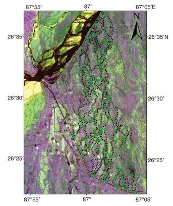
Figure 3. Landsat false color composite from 2 November 2005, from which paleochannel network (dashed lines) was extracted; stream junctions and bends are represented as nodes (green dots).
