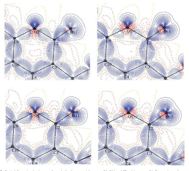
Figure 5. Static deformation density maps drawn in the plane containing atoms O1, O11, and C2, origin at atom O1. Contour intervals are at  $\pm 0.05$  e , positive and negative contours are in solid blue and broken red lines, respectively, and contour at zero level is shown as a broken yellow line.
