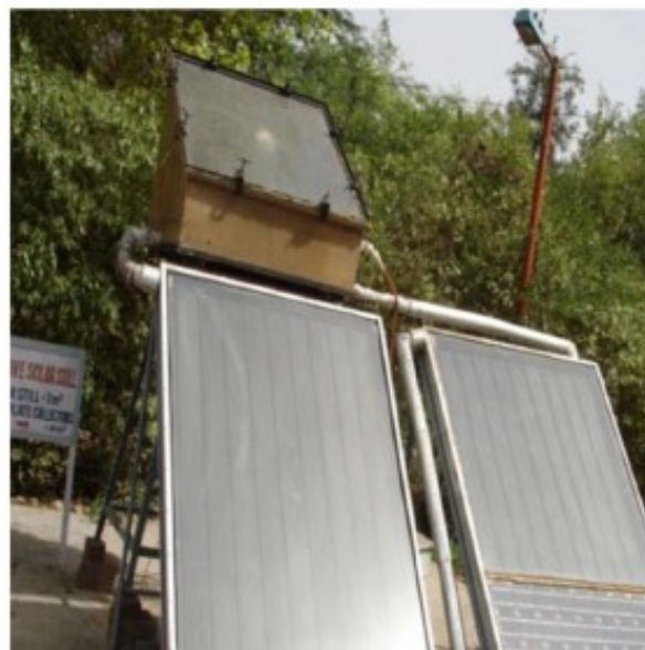
Figure 2. Hybrid (PV/T) active solar still [2]
