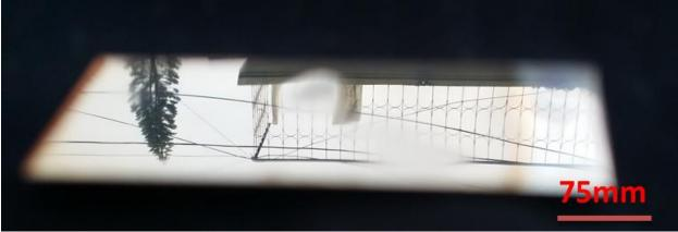
Figure 6 Photograph of as-deposited Cu-Sn alloy film showing a clear reflecting surface.
