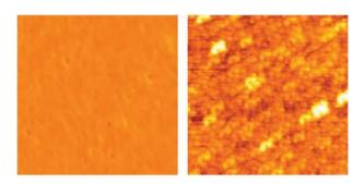
**Fig. 2** AFM images  $(0.5 \times 0.5 \,\mu\text{m}, \text{tapping mode})$  of substrate S3 before (left) and after (right) grafting of the fullerene monolayer.
