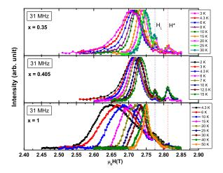
FIG. 9: Field sweep  $^{51}V$  spectra at 31 MHz. Vertical dotted lines at  $H_L$  and  $H^*$  (see text) are attributed to non-magnetic impurity phases.
