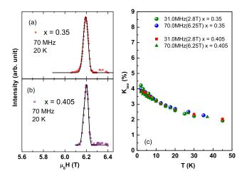
FIG. 3:  $^{51}$ V NMR spectra measured at 70 MHz and 20 K for (a) x = 0.35 and (b) 0.405, (c)  $K_{iso}$  for x = 0.35 and 0.405 sample as a function of temperature in two different fields.
