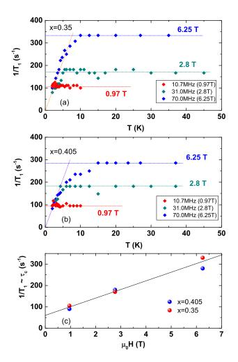
FIG. 4: (a) and (b):  $1/T_1$  vs. temperature T for x=0.35 and 0.405 at different fields, (c):  $\tau_c$  (correlation time of the spin fluctuations) as a function of applied field. The dotted and solid lines are for guide to the eye.
