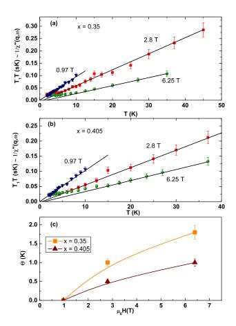
FIG. 5: (a) and (b): Tempereature dependence of  $T_1T$  at different fields for x=0.35 and 0.405, (c):  $\theta$  obtained from high temperature Curie-Weiss fits (straight lines) as a function of field for x=0.35 and 0.405. The curved lines are for guide to the eye.
