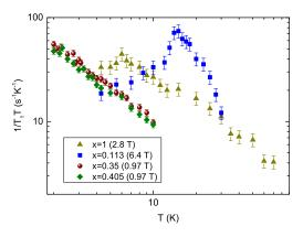
FIG. 12: Temperature depedence of  $1/T_1T$  at the respective lowest fields for each of the compounds. The figure indicates the doping evolution of electron spin-dynamics in  $\text{CeTi}_{1-x}V_x\text{Ge}_3$ .
