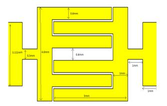
Fig. 1. Optimzed Design with dimensions
