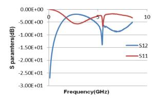
Fig. 4. Measured resturn loss and transmission coefficent of proposd design.
