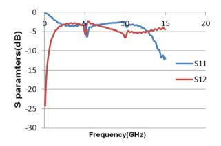
Fig. 2. S-parameters of the proposed design
