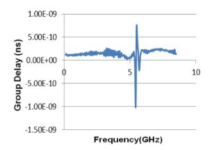
Fig. 5. Measured Group Delay of proposed design
