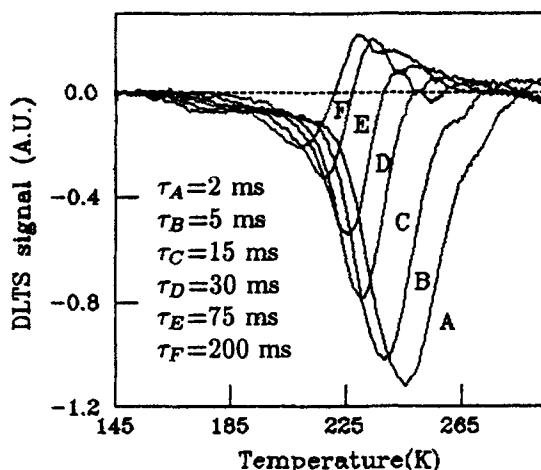
Figure 1. DLTS spectra of Si irradiated with  $\text{Ar}^+$  at dose  $1 \times 10^{14}\text{ cm}^{-2}$  showing negative peak for slower rate windows.
