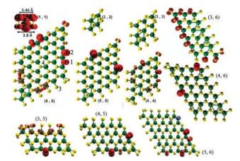
**Fig. 3** Spin density distribution in the (m,n) platelets. The green (yellow) balls correspond to Mo (S) atoms. Isosurface value of  $89 \times 10^{-3} \text{ e}^{-} \text{ Å}^{-3}$  is used.
