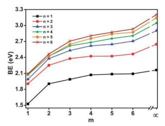
Fig. 2 BE of (m,n) parallelogram platelets along with the values for the corresponding  $MoS_{2+x}$  infinite nanoribbons. The values for (m,n) and (n,m)platelets are the same.
