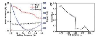
Fig. 6 (a) The total energy, and Mo-S as well as S(2c)-S(2c) bond distances for different lattice constants of  $(6, \infty)$  MoS<sub>2+x</sub> nanoribbons and (b) the magnetic moment as a function of S(2c)-S(2c) separation.
