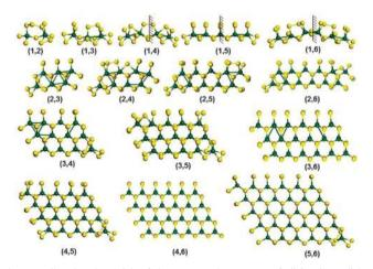
**Fig. 1** Ball-and-stick models of the optimized structures of all (m,n) parallelogram shaped platelets. The green (yellow) balls correspond to Mo (S) atoms. The structures for platelets with m = n are given in Fig. 3. Mirror symmetry is marked in some structures.
