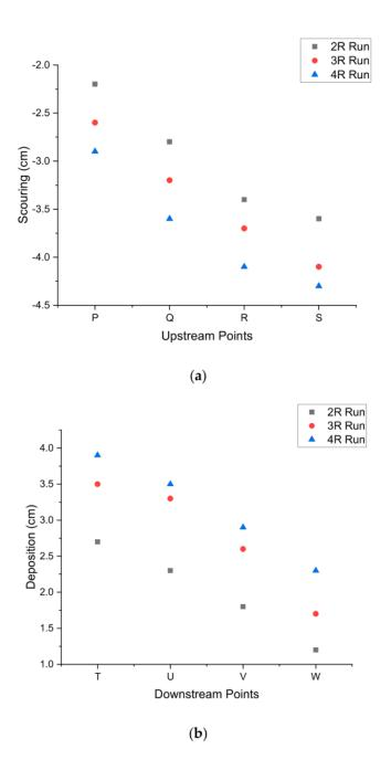
**Figure 5.** The scour profile for points upstream of mid-channel bar (**a**); the deposition profile for points downstream of mid-channel bar (**b**).
