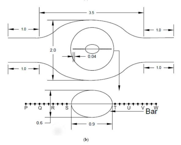
**Figure 1.** The model of braided bar constructed in the River Engineering lab at IIT Roorkee. (a) Photograph of mid-channel braided bar model; (b) the sketch of the bar model (all dimensions in meters).
