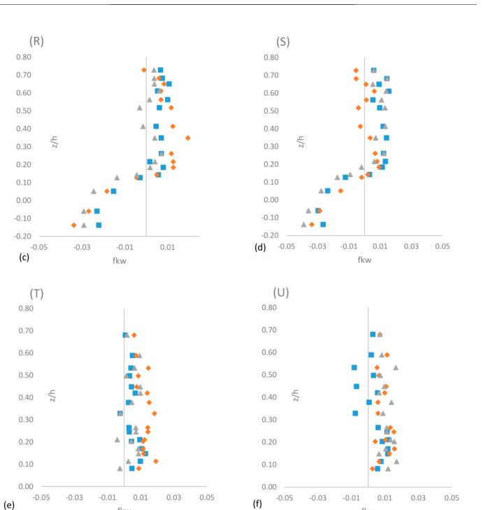
**Figure 9.** The depth-wise distribution of Fkw for -P- section (**a**), -Q- section (**b**), -R- section (**c**), -S- section (**d**), -T- section (**e**), and -U- section (**f**).
