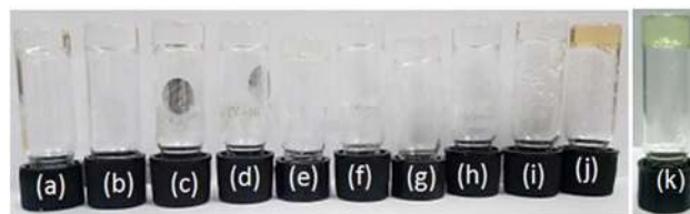
Figure 1 Organogels of (a) benzene (b) toluene (c) o-Xylene (d) m-xylene (e) p-xylene (f) mesitylene (g) 1, 2 dichlorobenzene (h) chlorobenzene (i) bromobenzene (j) Iodo benzene (k) diesel.
