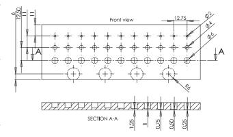
Figure 1: Test piece dimensions (all in mm.)
