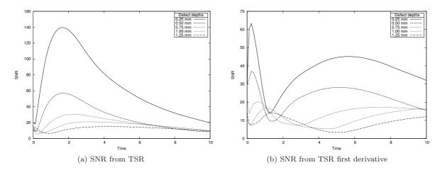
Figure 11: SNR obtained from pulsed TSR and its derivatives.
