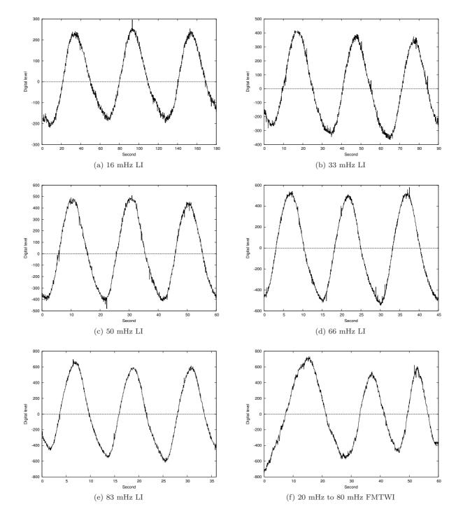
Figure 3: 3a-3e: Thermal oscillations obtained in lock-in thermography experiments on sound region at the frequencies indicated. 3f: FMTWI thermal oscillations observed on the sound region, indicating frequency increase with time.
