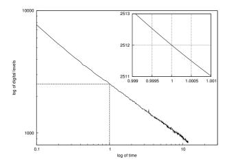
Figure 2: Plot of logarithmic temperature rise (digital level) against logarithmic time over sound region in pulsed thermography experiment. The inset plot zooms around t=1 second.
