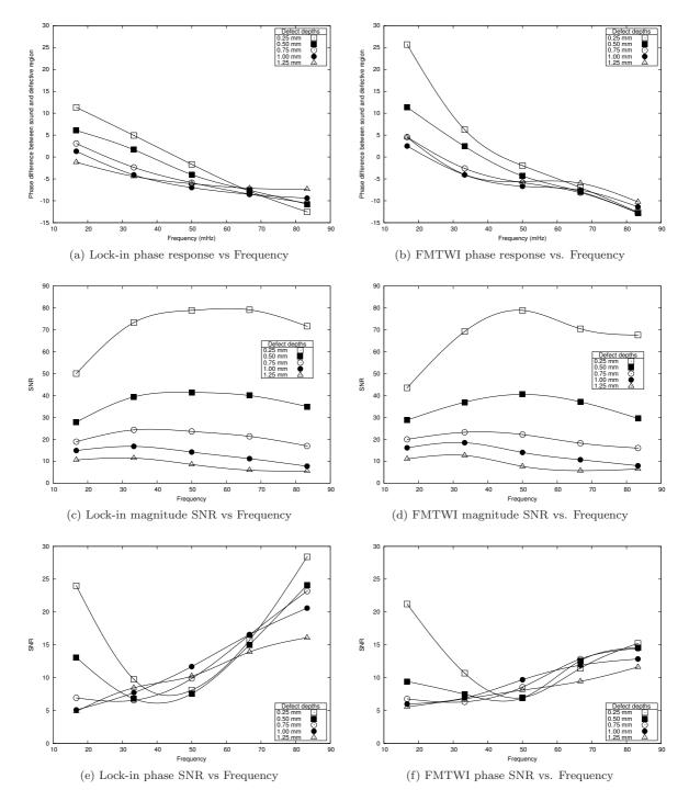
Figure 9: 9a & 9b: Phase difference between sound and defect regions analyzed as a function of frequency for lock-in and FMTWI tests for indicated defects. 9c & 9d: Plots of SNR observed in magnitude images of lock-in and FMTWI tests as a function of analysis frequency. 9e & 9f: Plots of SNR observed in phase images of lock-in and FMTWI tests as a function of analysis frequency.
