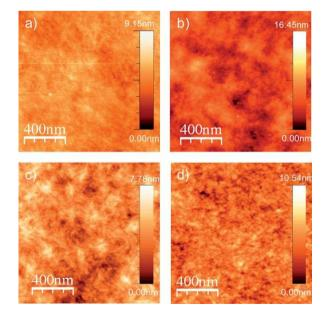
Fig. 5 AFM height images of a PDBFBT thin film ( $\sim$ 30 nm) without annealing (a) and annealed at 100 (b), 150 (c), and 200 °C (d) for 15 min under nitrogen.
