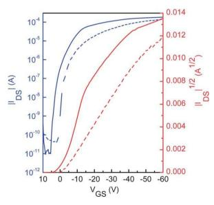
**Fig. 8** Transfer ( $V_{\rm DS} = -60$  V) characteristics of an OTFT device ( $L = 75 \ \mu m$ ;  $W = 4 \ mm$ ) with a PDBFBT thin film annealed at 100 °C measured in air (dotted lines) and under nitrogen after being re-heated at 100 °C for 30 min (solid lines). The calculated mobility in the saturation regime is 0.17 cm<sup>2</sup> V<sup>-1</sup> s<sup>-1</sup> measured in air and 0.74 cm<sup>2</sup> V<sup>-1</sup> s<sup>-1</sup> measured under nitrogen after being re-heated.
