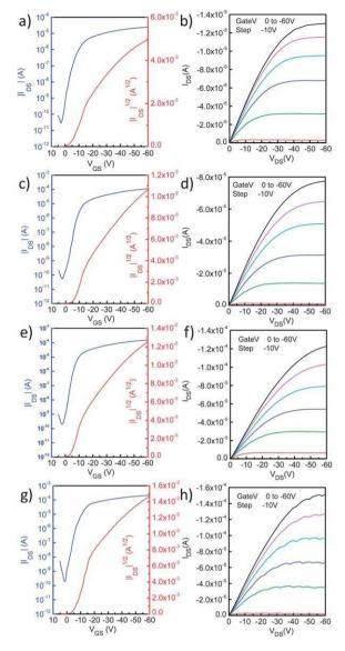
Fig. 7 Output ( $V_{GS} = 0$  V to -60 V) and transfer characteristics of OTFTs with a PDBFBT thin film without annealing (a and b), annealed at 100 °C (c and d), 150 °C (e and f), and 200 °C (g and h) for 15 min under nitrogen ( $L = 125 \mu$ m; W = 4 mm).
