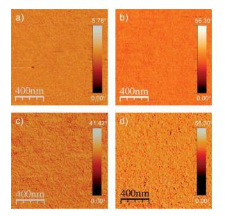
Fig. 6 AFM phase images of a PDBFBT thin film ( $\sim$ 30 nm) without annealing (a) and annealed at 100 (b), 150 (c), and 200 °C (d) for 15 min under nitrogen.
