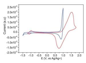
Fig. 3 Cyclic voltammograms of a PDBFBT thin film (red lines) and a PDQT<sup>8</sup> thin film (blue lines) showing the first oxidative and reductive cycles at a scan rate of 100 mV s<sup>-1</sup>. The electrolyte was 0.1 M tetrabutylammonium hexafluorophosphate in anhydrous acetonitrile.
