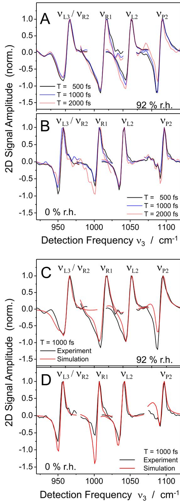
FIG. 4. Cuts through the 2D spectra at  $T = 500, 1000,$  and  $2000$  fs for (a) 92% and (b) 0% r.h. along the anti-diagonal axis in the 2D frequency frame with a comparison to the calculated 2D spectra at  $T = 1000$  fs for (c) 92% and (d) 0% r.h. The anti-diagonals cross the diagonal  $\nu_1 = \nu_3$  at a characteristic frequency position for the maximum of the corresponding backbone mode.
