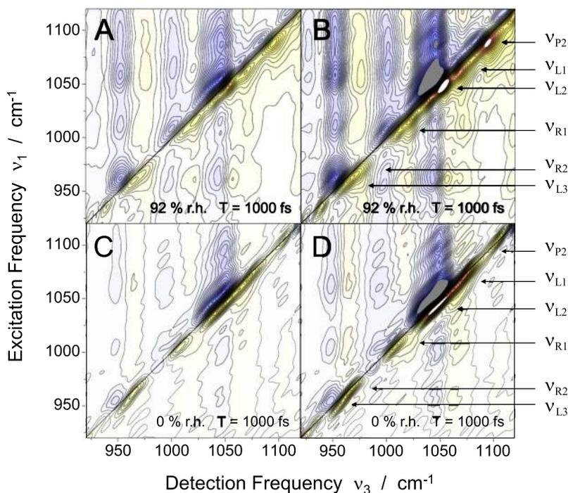
FIG. 3. 2D spectra of the DNA oligomers at (a) 92% r.h. and (c) 0% r.h. The spectra were recorded at a population time of  $T = 1000$  fs. Positive and negative signals are plotted as yellow-red and blue contours, respectively. The signals are normalized to their maximum values, the amplitude changes by 5% between neighboring contours lines. (b) and (d) display the same spectra normalized to half of the maximum in the absolute signal level for comparison of the low-contrast features.
