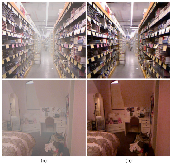
Fig. 6. Results of the proposed method when tested on two sample images taken from the NYU depth V2 dataset. (a) the hazy images and (b) the clear image dehazed by the proposed method. The proposed model, due to the inclusion of SSIM loss, provides more closer results to the ground truth, by preserving the minute texture information (especially in the second image).
