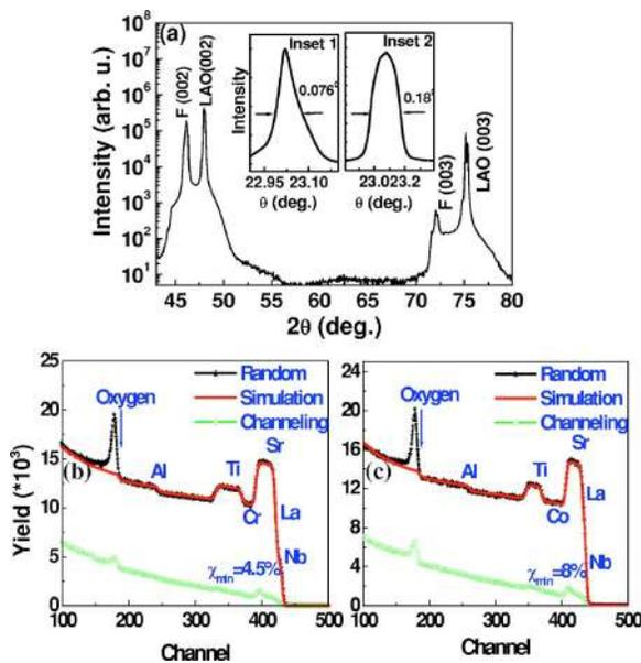
FIG. 1. (Color online) (a) A typical  $\theta$ - $2\theta$  XRD pattern for 2%MTE, Nb:STO thin films on  $\text{LaAlO}_3$  (001). Peaks labeled "F" correspond to the film. Inset 1 shows the XRD rocking curve for a thin film with chromium doping. Inset 2 shows the rocking curve for a cobalt doped one. [(b) and (c)] 3.05 MeV  $\text{He}^+$  Rutherford backscattering (RBS) random simulation and channeling spectra for the 2%Cr, 0.5%Nb doped STO and 2%Co, 0.5%Nb doped STO thin films, respectively.
