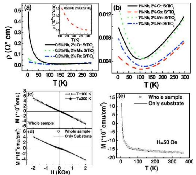
FIG. 3. (Color online) [(a) and (b)] Temperature dependence of resistivity for these thin films: 2%MTE, 0.5%Nb doped STO and 2%MTE, 1%Nb doped STO, respectively. (c) Typical  $M$  vs  $H$  for one thin film (including substrate) at 300 and 100 K. (d) Comparison of  $M$ - $H$  for one sample with a heated pure substrate at 15 K. (substrate area unity:  $\text{emu}/\text{cm}^2$ ). (e) Comparison of  $M$ - $T$  for one sample with a heated pure substrate at an applied field of 50 Oe.
