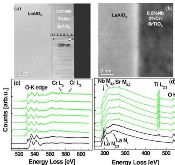
FIG. 2. (Color online) (a) Cross sectional TEM image at large length scale of the 2%Cr, 0.5%Nb doped STO film grown on  $\text{LaAlO}_3$  (001) substrate. (b) High resolution TEM image for the interface between the film and substrate [(c) and (d)] EELS line scans across the cross section of the sample.
