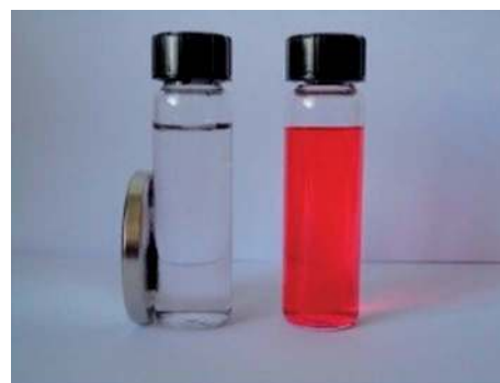
Fig. 8 Photograph of the fuchsine solution ( 20 \text{ mg L}^{-1} , right) and the solution after adsorption with the G/ \text{Fe}_3\text{O}_4 adsorbent for 1 h and separation with a magnet (left). Reproduced with permission from ref. 239.
