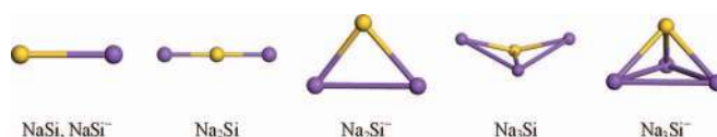
FIG. 1. The lowest energy structures of neutral \text{Na}_n\text{Si} and anionic \text{Na}_n\text{Si}^- clusters ( 1 \leq n \leq 3 ). Yellow balls are for silicon and blue balls for sodium atoms.
