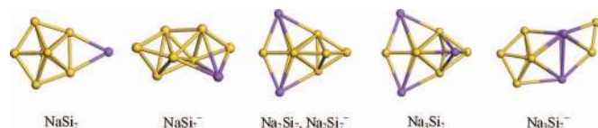
FIG. 7. The lowest energy structures of neutral \text{Na}_n\text{Si}_7 and anionic \text{Na}_n\text{Si}_7^- clusters ( 1 \leq n \leq 3 ). Yellow (blue) balls represent silicon (sodium) atoms.
