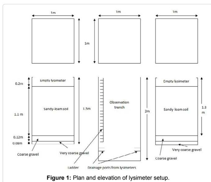
Figure 1: Plan and elevation of lysimeter setup.
