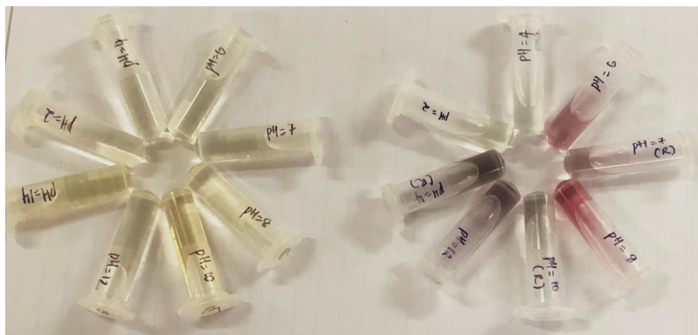
Fig. 6. Effect of pH on QGDs (left) and QGD-Au hybrid particles (right).
