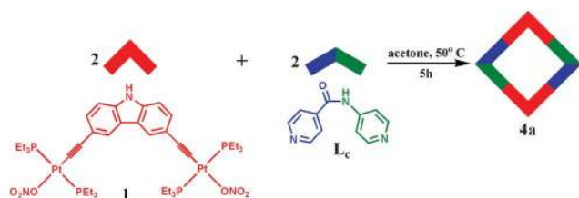
Scheme 3 [2 + 2] self-assembly of molecular rhomboid 4a via an organometallic 90^\circ acceptor, 1 , and a linear flexible ambidentate ditopic donor ( L c ).
