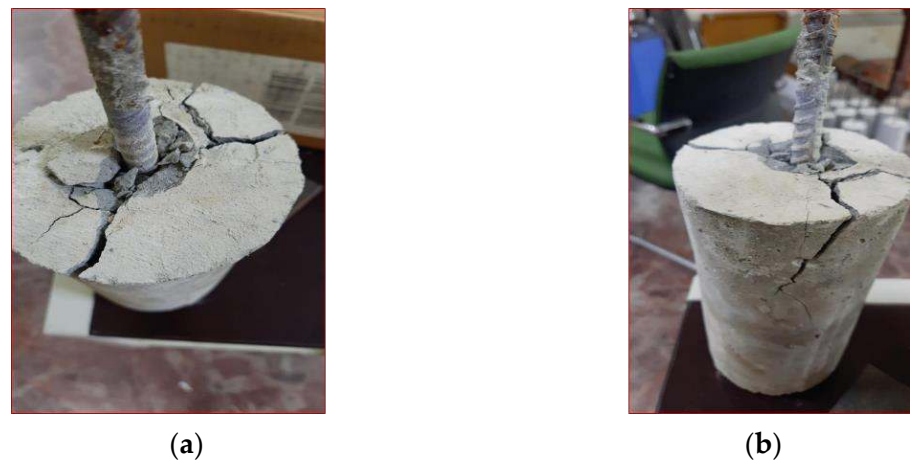
Figure 12. Different views of failure mode (a) Top, (b) Side.
