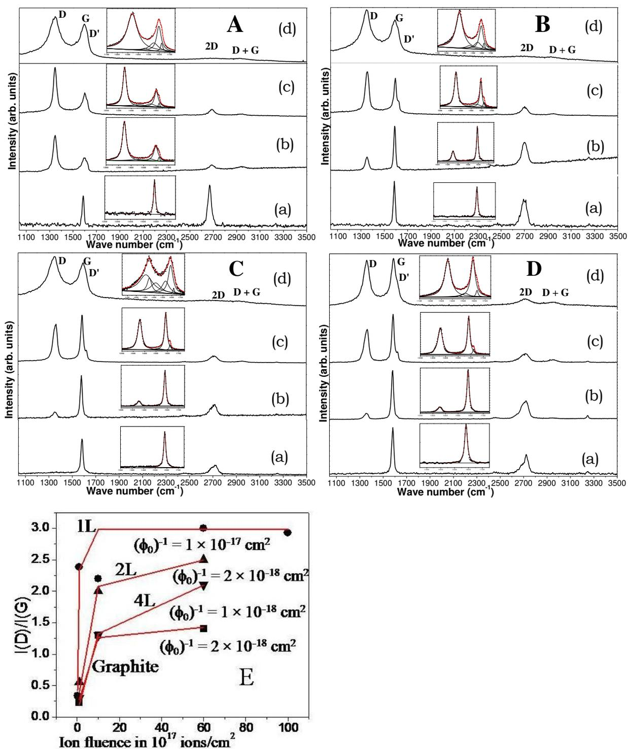
Fig. 3- Panel A-Raman spectrum from (a) pristine monolayer graphene and the same sample irradiated at fluences of (b)  $1 \times 10^{17}$  ions/cm<sup>2</sup>, (c)  $1 \times 10^{18}$  ions/cm<sup>2</sup> and (d)  $6 \times 10^{18}$  ions/cm<sup>2</sup>, panels B, C and D correspond to the same for a 2 layer graphene, 4 layer graphene and Graphite
