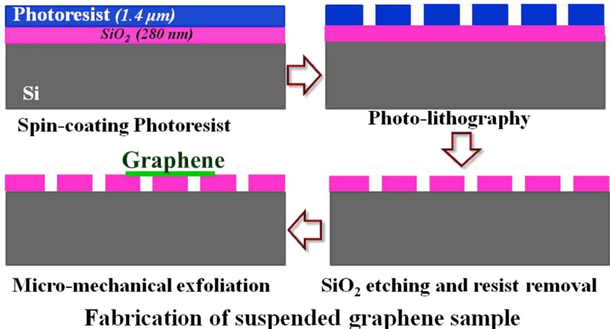
Fig. 1. Schematic of the fabrication of suspended graphene samples.
