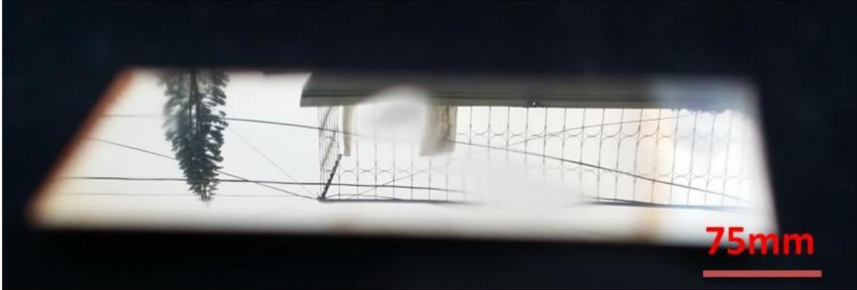
Figure 6 Photograph of as-deposited Cu-Sn alloy film showing a clear reflecting surface.
