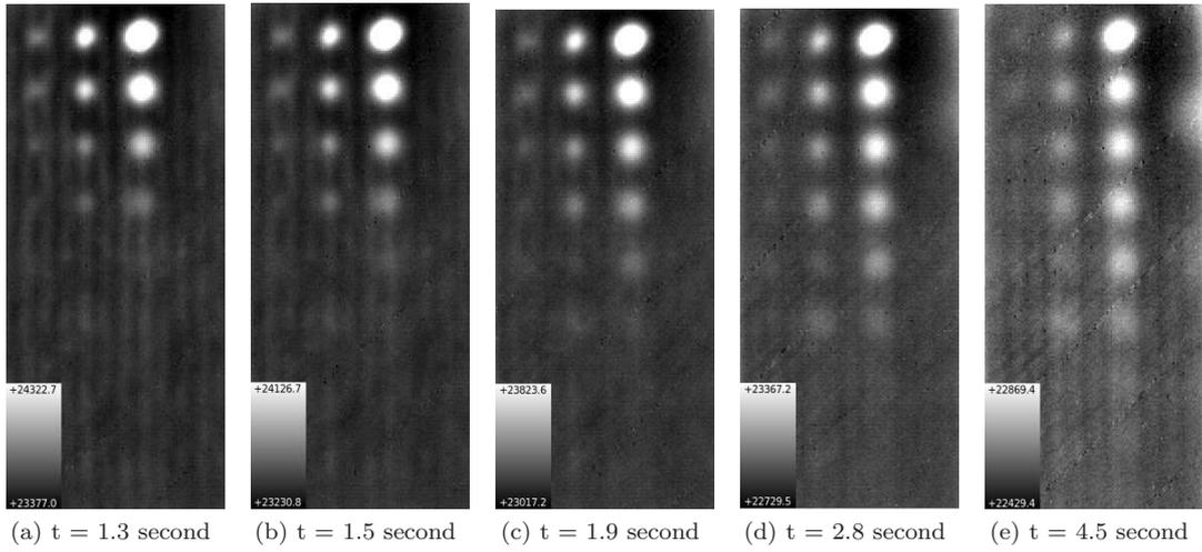
Figure 5: Pulsed thermography frames with maximum SNR for each of the 6 mm diameter defects mentioned in table 4. The scale bar indicates the range of digital levels covered by the thermal image.
