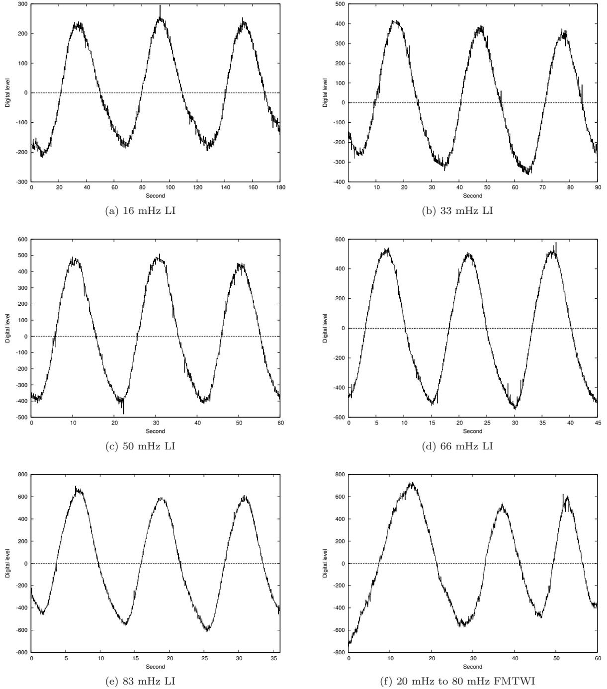
Figure 3: **3a-3e**: Thermal oscillations obtained in lock-in thermography experiments on sound region at the frequencies indicated. **3f**: FMTWI thermal oscillations observed on the sound region, indicating frequency increase with time.
